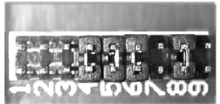
9 position jumper (This pushbutton is set for Ding Dong Chime since 7=off, 8=on, and 9=off.)
